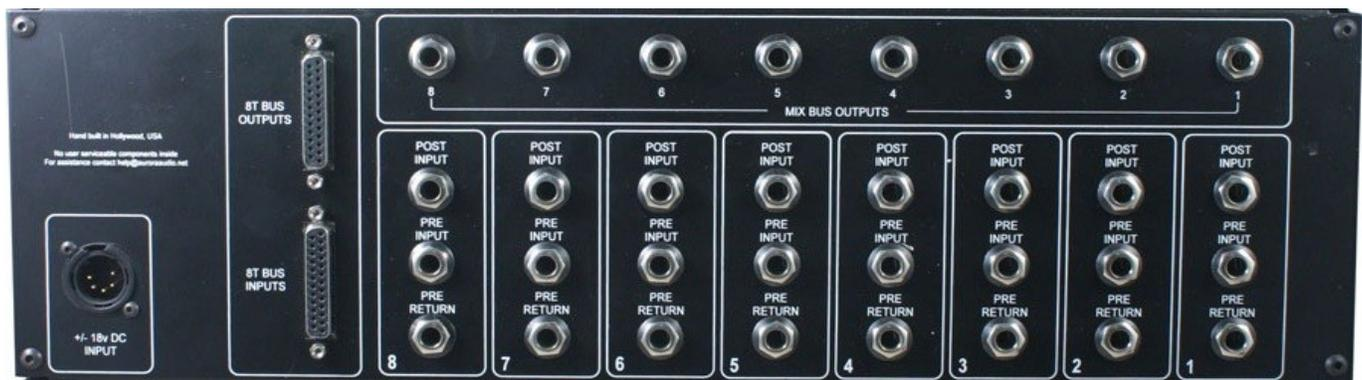
There are two inputs per channel marked "PRE INPUT" and "POST INPUT". The PRE INPUT normally wires to the GTM822's channel pre-fade insertion send jack and the PRE RETURN jack is in parallel with the PRE INPUT jack and intended as a loop through to a patch bay so that the GTM822's insertion path is retained. The POST INPUT is wired to the GTM822 channel output XLR.
